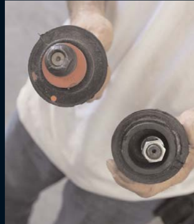
Here are the installed pieces (out of a bike) to show even a layman how much more support the Glide-Pro offers the end of the shaft compared to the stock arrangement.
