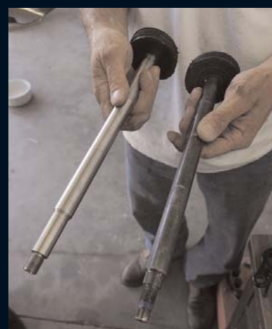
Here's the original pivot shaft (right) and the Glide-Pro unit (left). Notice the longer shoulder area at the end, which is where the polyurethane bushings ride.
