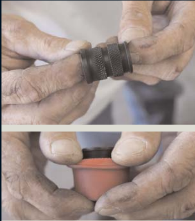
The “walking” problem was solved in later versions by adding knurling and grooves to lock in the rubber. The pressure-molded bushing is now sturdy enough to resist even a determined attempt to dislodge it.
