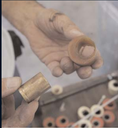
Glide-Pro designer Jake Ore shows us an early prototype of the Glide-Pro with a soft durometer rubber bushing and smooth inner sleeve. The sleeve had a tendency to “walk” in this version. Several of the subsequent versions are shown in the background.
